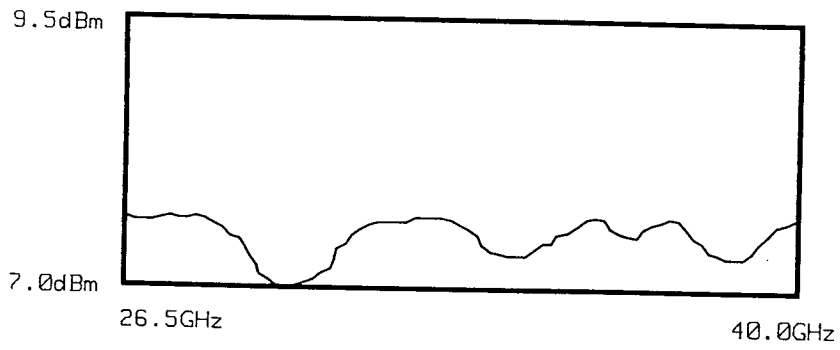
Figure 2-8. Power Flatness Response (26.5 to 40.0 GHz)
